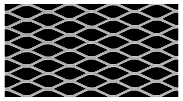
LW Pitch:38.10mmStrand Width:2.50mmSW Pitch:14.00mmThickness:1.20mmWeight:3.37 kg / m2Open Area:64%
